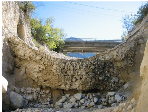
Figure 1. Testing of the flexible system in the Illgraben canal, Switzerland 2006. Approximate retention volume 1000\text{m}^3
